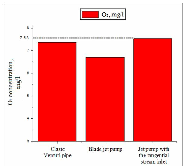
Fig.9. Solubility of oxygen in water-jet ejectors
