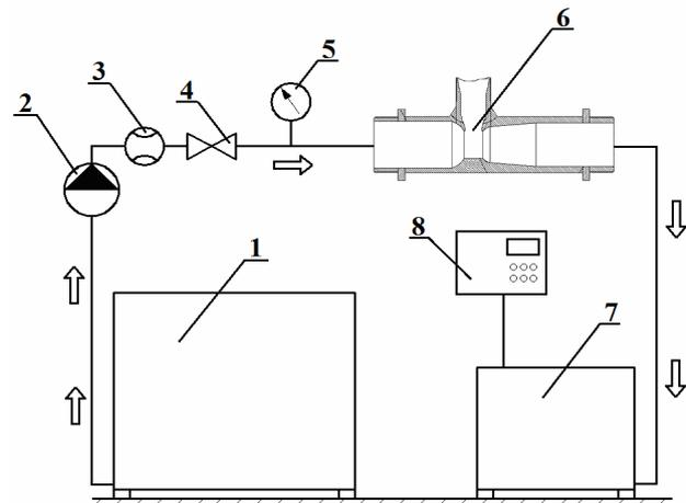
Fig. 5. Experimental stand with Venturi pipe: 1 – water capacity; 2 – water pump; 3 – flow meter; 4 – adjustable damper; 5 – pressure meter; 6 – the classic Venturi pipe; 7 – capacity; 8 – oksimeter
