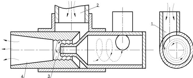
Fig. 3. Scheme of the jet pump with the tangential stream inlet: 1 – stream inlet; 2 – intake; 3 – mixing chamber; 4 – diffuser
