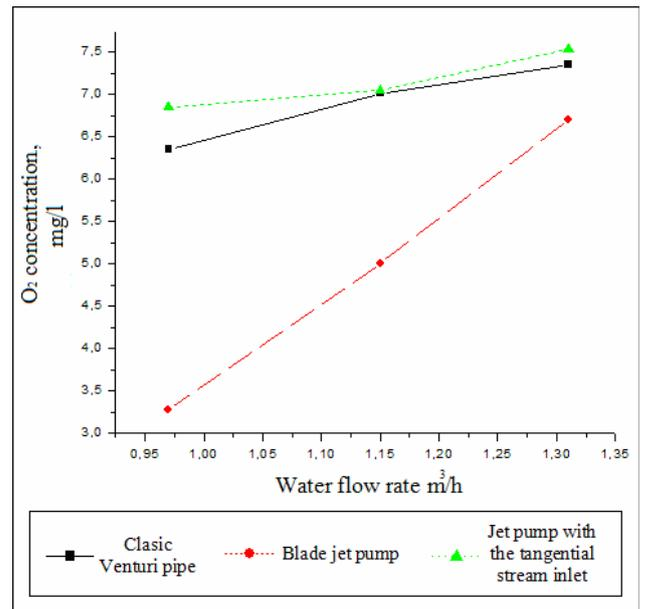
Fig.8. Solubility of oxygen in water-jet ejectors according to water flow rate
