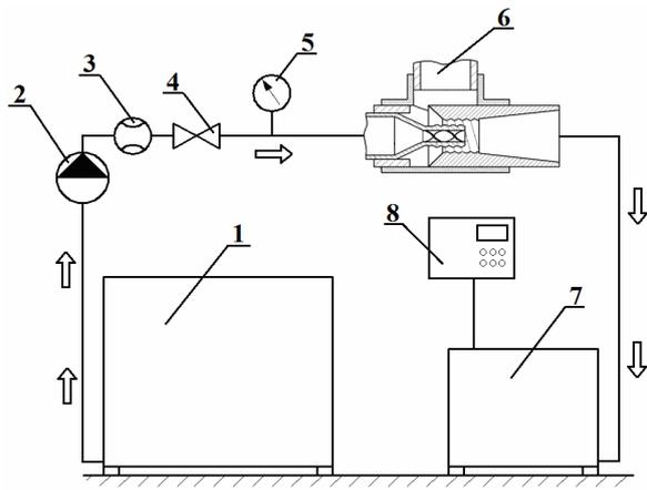
Fig.6. Experimental stand with blade jet pump: 1 – water capacity; 2 – water pump; 3 – flow meter; 4 – adjustable damper; 5 – pressure meter; 6 – the blade jet pump; 7 – capacity; 8 – oximeter
