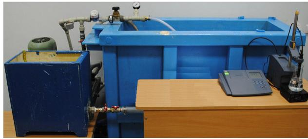
Fig. 4. The experimental stand investigation on the solubility of oxygen in water-jet ejectors.
