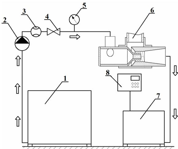
Fig.7. Experimental stand with modified jet pump: 1 – water capacity; 2 – water pump; 3 – flow meter; 4 – adjustable damper; 5 – pressure meter; 6 – the jet pump with the tangential stream inlet; 7 – capacity; 8 – oximeter
