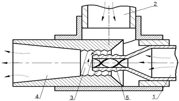
Fig. 2. Scheme of blade jet pump: 1 – stream inlet; 2 – air intake; 3 – mixing camera; 4 – diffuser; 5 – twisted blades
