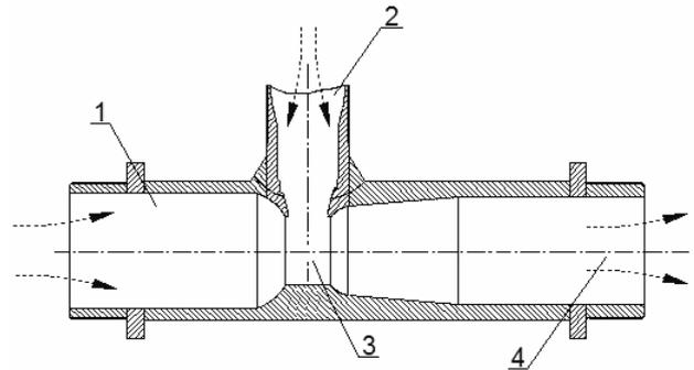
Fig.1. The classic Venturi pipe: 1 – stream inlet; 2 – air intake; 3 – mixing camera; 4 – diffuser
